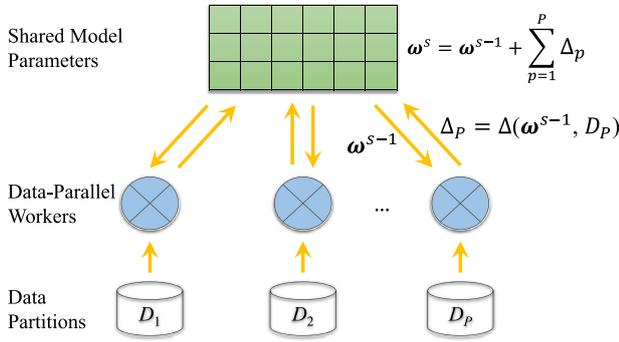
Fig. 1. Illustration of data parallelism and parameter server topology.
